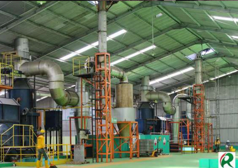
Project Name: Hazardous Waste Incinerator Type: Reciprocating System Capacity: 300 Kg per Hour Scope: Engineering Design, Fabrication and Installation Year Installed: 2013 Customer: Hazardous Waste Treatment Plant - East Java
