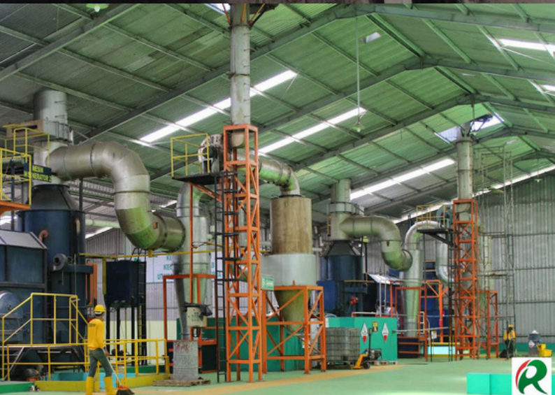
Project Name: Hazardous Waste Incinerator Type: Reciprocating System Capacity: 300 Kg per Hour Scope: Engineering Design, Fabrication and Installation Year Installed: 2013 Customer: Hazardous Waste Treatment Plant - East Java
