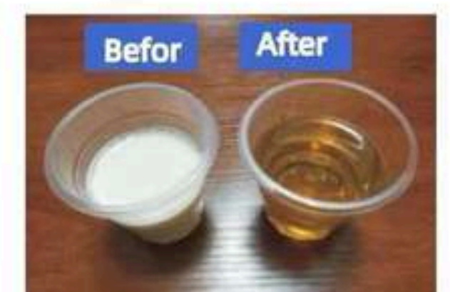
Comparison of emulsified hydraulic oil filtration
